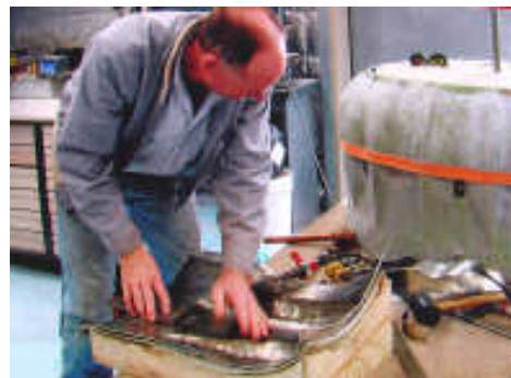
A: Kevin building a new engine cowling B: stripped to the bare metal, this was a big job.
