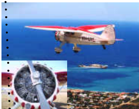
You need a step ladder VH-UXL stands pretty tall powered by a 300HP Lycoming R680 which still has a half life to run.
