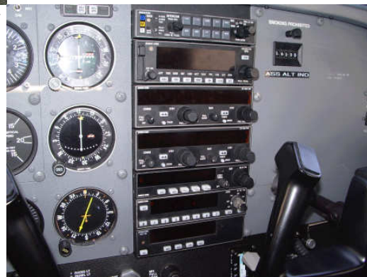
VH-KOT has the King Nav 2 IFR package, two Com/Nav radios, ADF, Transponder, TSO GPS, and Auto Pilot
