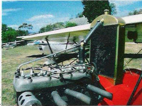
1928 Model A Ford engine with original rods, cam and crank. New bearings, Pistons and oil system.
