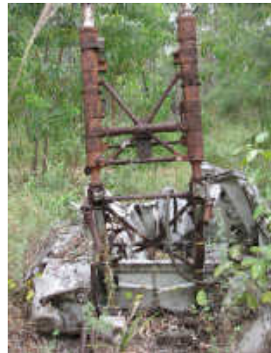
Starboard undercarriage of the Beaufort. It crashed after the port undercarriage collapsed on touchdown.
