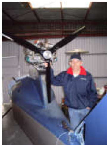
Kyle with the Rotax 912 ULS 100hp version with ground adjustable prop
